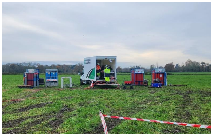
Figure 3 – NPL controlled release system being used to generate traceable emissions of CO 2
