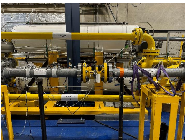
Figure 1 – Testing a turbine meter at FORCE Piston Prover
