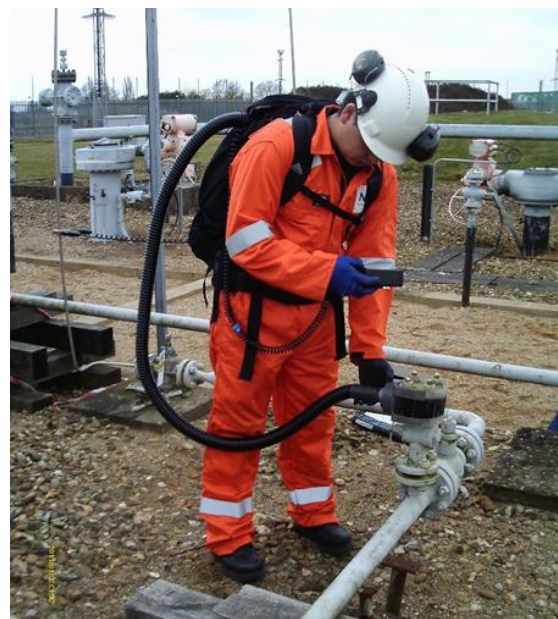
Figure – Hi-Flow sampler used for leak quantification
