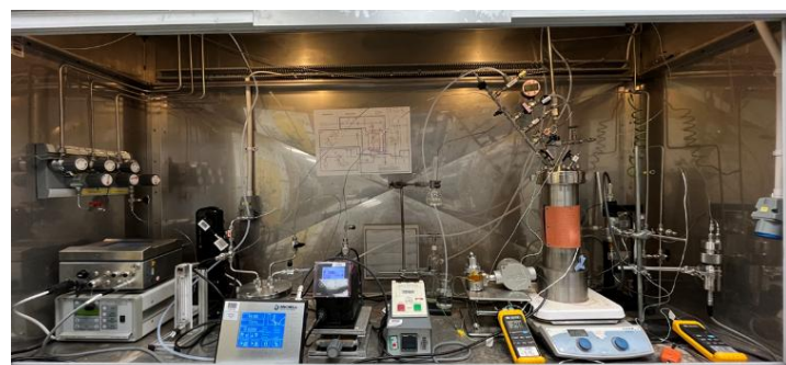
Figure – New facility for corrosion testing of pipeline steel in impurity-containing dense phase CO 2 environment.
