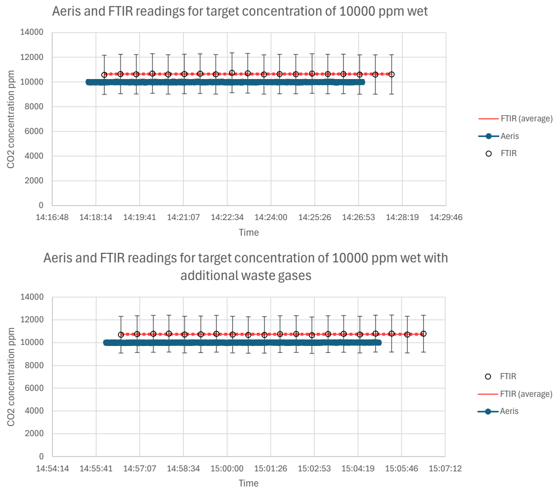
Figure 6. Aeris and FTIR measurement results for a target concentration of 10000 ppm alone and with additional waste gases within a simulated wet flue gas matrix, and associated uncertainties.
