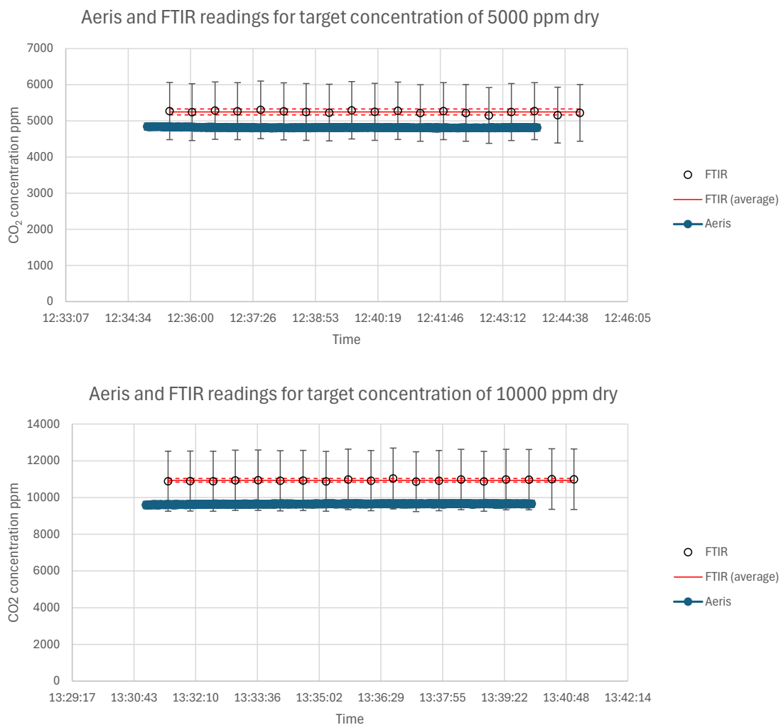
Figure 5. Aeris and FTIR measurements for target concentrations of 5000 and 10000 ppm within a dry flue gas matrix and associated uncertainties.
