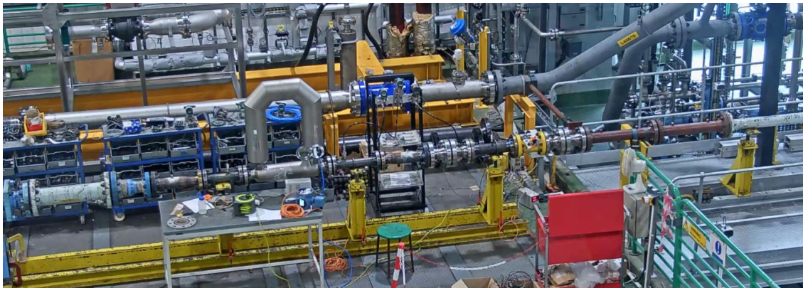
Figure 4 – Picture of the 4-inch turbine and Coriolis meter installed at NEL. The meters are installed in series with the turbine upstream of the Coriolis meter. The flow is from right to left.
