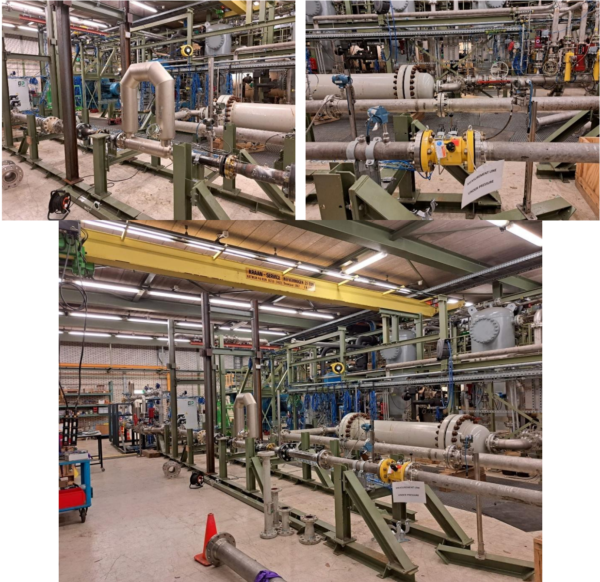
Figure 5 - Pictures of the 4-inch turbine and Coriolis meter installed at DNV. The meters are installed in series with the turbine upstream of the Coriolis meter. The flow is from right to left.
