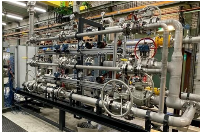
Figure 2 - Schematic (top) and picture (bottom) of the reference section of the All Gas Flow Loop Groningen (AGFLG) test facility at DNV. From the right, the gas flows first through the Meters Under Test (MUT), then through the reference Coriolis meters, the reference turbine meters, and the reference Critical Flow Venturi Nozzles.
