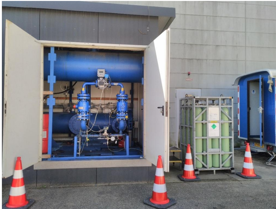
Figure 16 - A picture of the SICK FL550 installed on the GOPP for calibration with CO 2 and Natural gas
