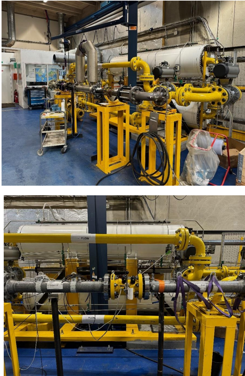
Figure 6 - Pictures of the 4-inch turbine (bottom) and Coriolis meter (top) installed at FORCE. The meters are not tested in series like in the other facilities due to length constraint.
