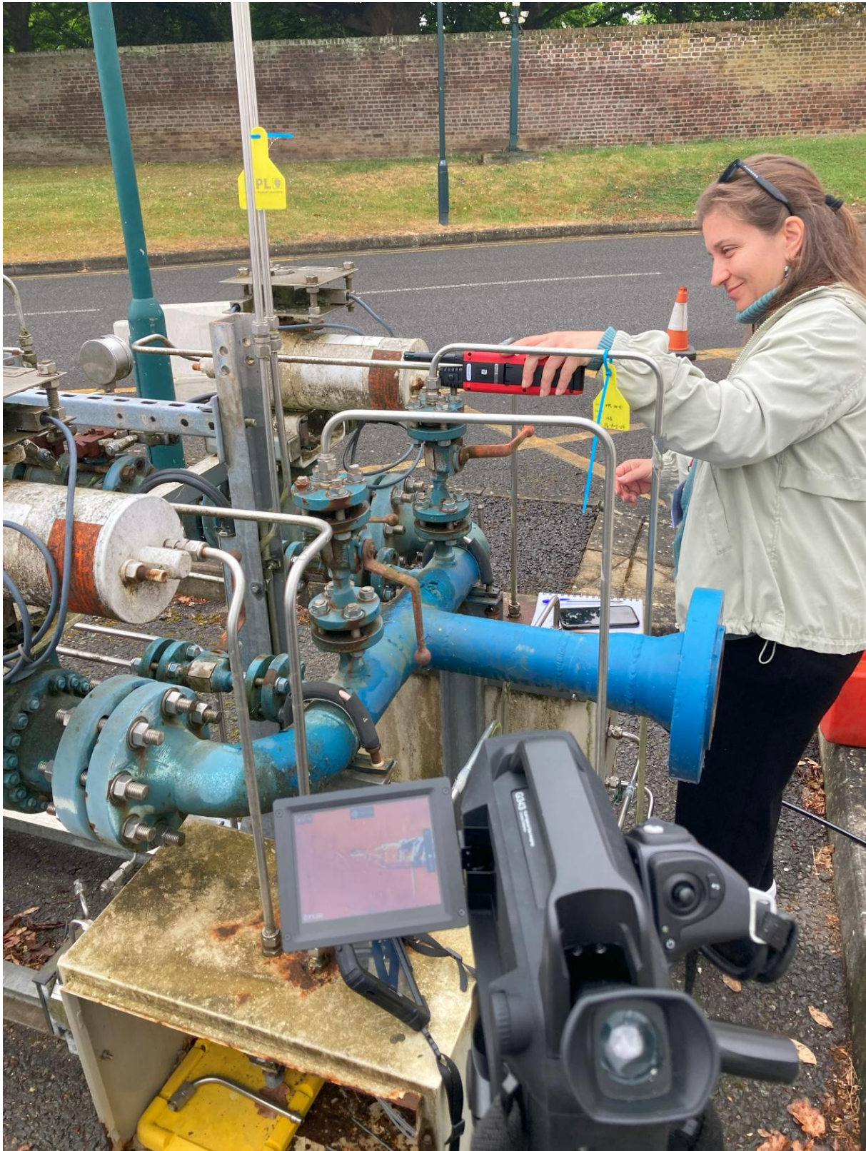
Figure 6: Leak detection using an OGI camera and Sefram device on a test rig.
