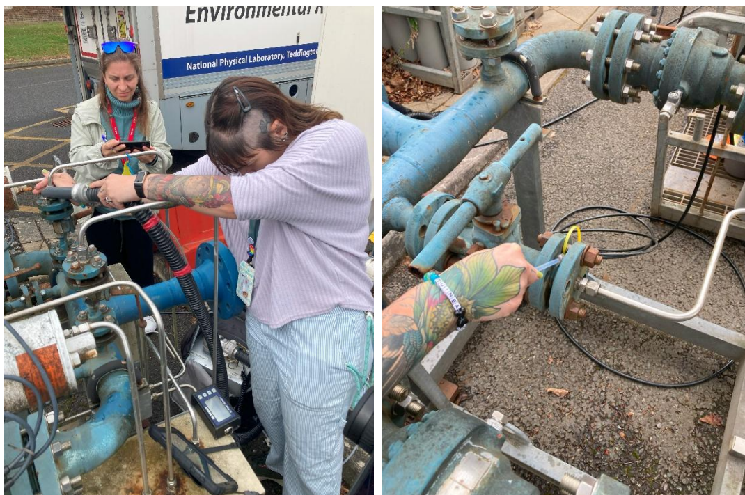
Figure 7: Leak detection Aeris and Aeris/Hi-Flow combination on a test rig. Aeris/Hi-Flow measurement of leaking compression fitting (left) and Aeris measurement of leaking flange (right)
