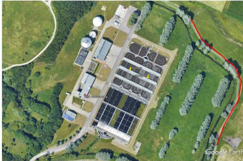
Figure 14: The measured wastewater treatment plant (left) including the measurement road (red line) and the tracer gas placement (orange marks).
