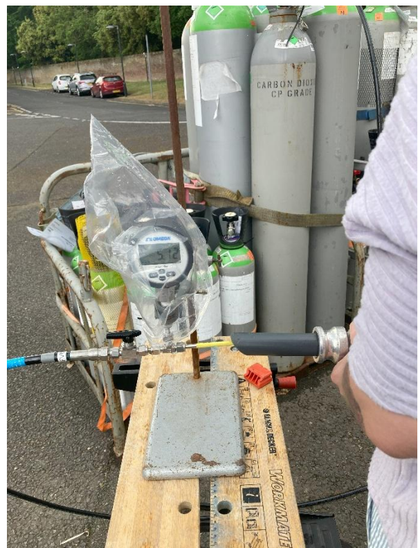
Figure 8 (left): Set up of the calibrated orifice in test 1 sampling directly from the source & figure 9 (right) sampling with the fugitive emissions leak rig
