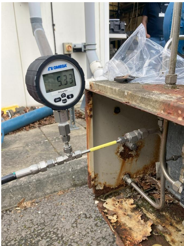
Figure 8 (left): Set up of the calibrated orifice in test 1 sampling directly from the source & figure 9 (right) sampling with the fugitive emissions leak rig
