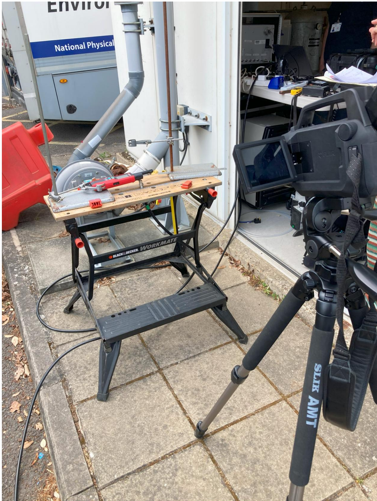
Figure 5: Leak detection from a tube outlet using an OGI camera and Sefram device.
