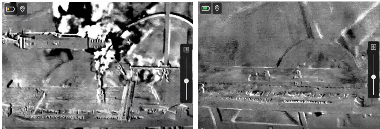
Figure 10: Still images of CO 2 controlled releases taken with G320 OGI camera for: a high leak rate (left, 5000 mL/min) and at low leak rate (right, 5 mL/min)
