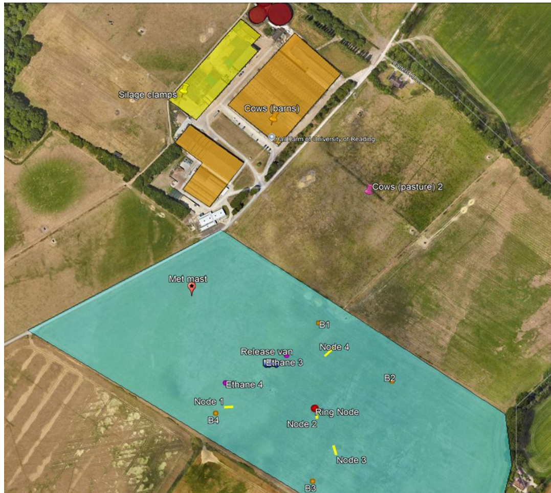
Figure 3: Configuration of the controlled release experiments at CEDAR showing location of Ring Node.
