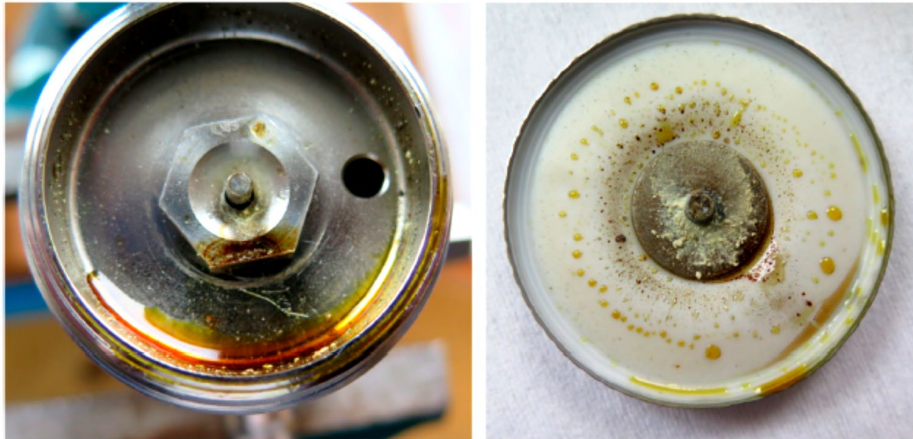
Figure 10: Products precipitated inside the heated regulator body (left) and on regulators diaphragm (right) [5]. Green/yellow solids on the right is elemental sulphur.
